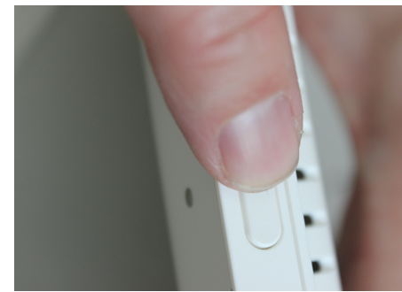
Push and hold the standby button on the side of the panel for 3 seconds
