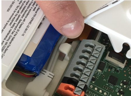
Route the wire behind the retainer clip
