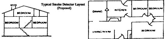
In homes with more than one sleeping area a smoke detector should be provided to protect each area. Smoke detectors shall be located between the sleeping area and the rest of the house. NOTE: Refer to N.F.P.A. 874 Appendix B1.1 through B-10.
